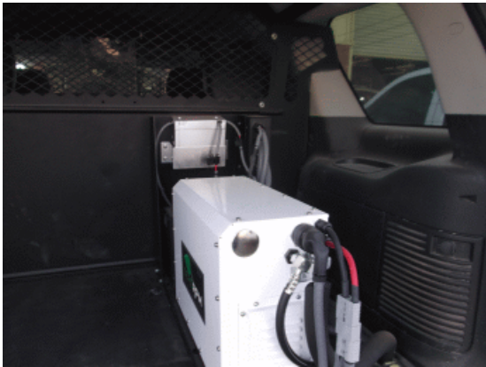
Figure 6: ZeroRPM IMS 60 (left) and IMS 100 (right) installed in load area of Chevrolet Tahoe. Courtesy of U.S. Border Patrol.
