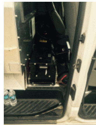
Figure 5: Battery system installed behind front seats of paddy wagon van. Courtesy of City of Dallas.
